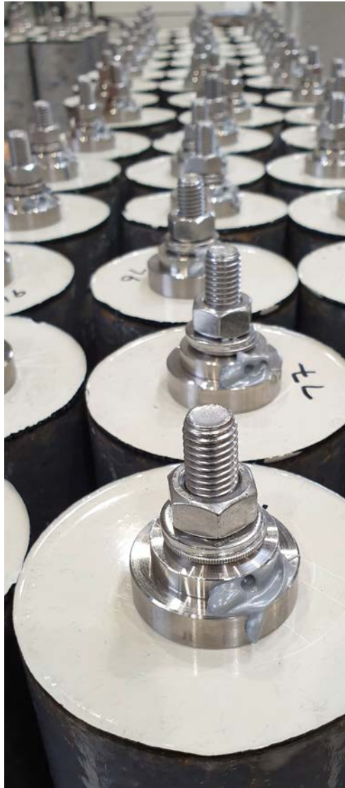
Anchoring systems have to be tested in elaborate test series. Here you can see test cylinders being sampled from a coated concrete surface.
